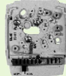
3 wire subbase with Heat/Cool switch. For use with 3WT thermostat. When set for "Heat", damper will open on temperature fall. When set for "Cool", damper will open on temperature rise. \*Not for use with Zone systems. Terminals: R, W, Y.
