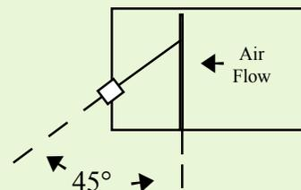
3-Set all thermostats so that all zones call for heat. Relocate the pressure relief damper counterweight to a point which keeps damper closed without flutter.
