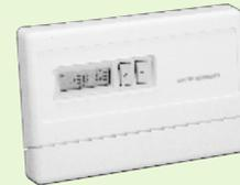
5 + 2 programming. Auto Changeover Electronic clock thermostat. Heat - Off - Cool & Fan Auto - On switches. Battery powered. 24 volts not needed at thermostat. Terminals: R, W, Y, G, B, O. Use on all SMZ Panels.
