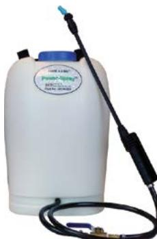
**Power-Spray™ Applicator Kit:** This unit holds a little over four gallons and can be carried on the operator's back. A 4-speed pump controls the volume of lube applied. The pump is operated by a re-chargeable battery with about eight hours usage time. The unit comes complete with re-charger and a spare battery. The outlet hose also leads to a quick disconnect coupling.
