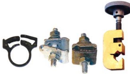
Temporary Lashing Clamps (62560-000) secure lashing wire to a termination point in mid-span or at a pole. The clamp is machined from solid cold drawn brass with a plated screw to eliminate corrosion if inadvertently left on strand for an extended period.
