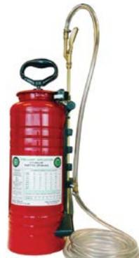
**Manual Applicator Kit:** A manually pressurized spray tank with a pressure gauge allows the user to monitor the amount of lube being sprayed onto the cable via the included hand-held wand, or any of DCD's products fitted with a quick connect spray nozzle. Different pressures allow different volumes. A manual shut-off valve leads to a quick disconnect coupling.
