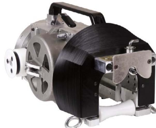
Magazine style doors provide easy loading of metallic or non-metallic lashing wire. Front and rear rollers made from Delrin allow smooth passage of cable and also protect your cable from damage. A simplified rear gate design with quick release mechanisms allows for efficient adjustment of the rear roller.
