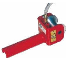
**Duct Entry Guide (32500 series):** This product fits right into the duct opening and has a roller that the cable must pass over. The unit is fitted with a spray nozzle that when hooked up, places the lubricant right onto the cable as it passes under the nozzle.
