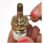
Lower the handle stop and replace the c-clip
