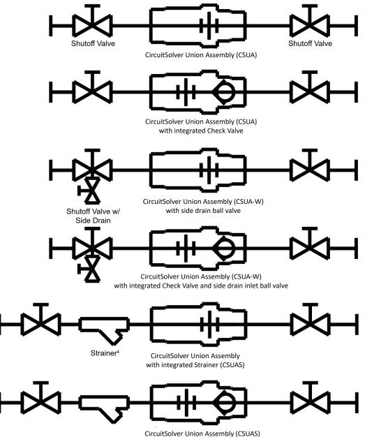
circuitSolver Union Assembly (CSUAS) with integrated Check Valve and Strainer
