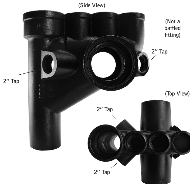
Part No. SV-1739D Vented Closet Cross with 2" 45° Taps (Designed for use above the floor)
