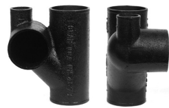
Part No. NH 457 Vented Closet Tee with 2" Top Vent (Left Hand or Right Hand; Designed for use below the floor; Fitting does not require a baffle.)
