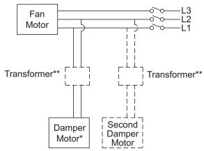
For 3-Phase, damper motor voltage should be the same between  $L_a$  and  $L_a$ . For single phase application, disregard  $L_a$ .
