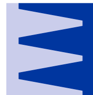
Dryseal pipe threads, wrench tight. Tightly seals all thread surfaces, providing a positive seal.
