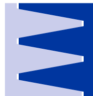
Regular pipe threads, hand tight. Only seals joints on the sides of the threads, allowing spiral leakage
