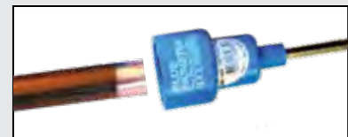
Fully retract fitting brush into the housing to clean O.D. of copper tube.
