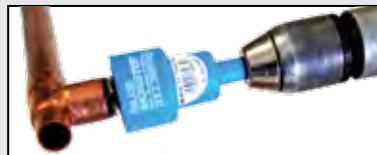
Push brush through the housing to clean I.D. of copper fittings.
