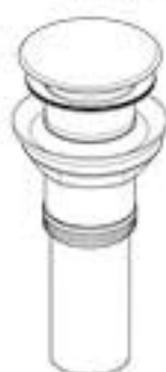
RP72413▲ Push Button Drain less overflow holes
