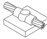
Type CAHE Through conductor to top of horizontal CAST IRON pipe or flat surface.
