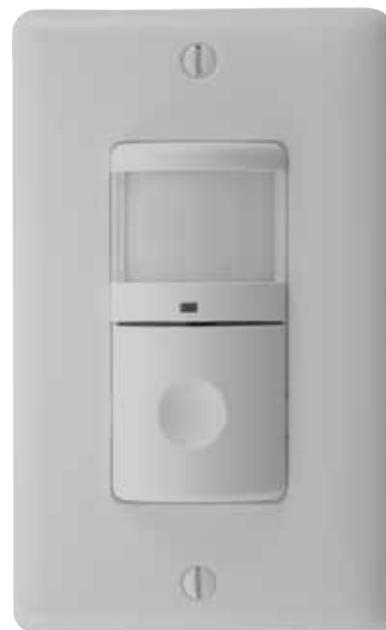
Hubbell WS/ATP series wall switches combine PIR sensing technology, photocell control, and Hubbell's patented three wire method to provide the perfect light switch replacement solution. These sensors do not require a neutral connection and they have no minimum load requirements. The WS series has manual timer adjustment while the ATP series incorporates Hubbell's patented adaptive technology to automatically set timing and eliminate manual adjustments.
