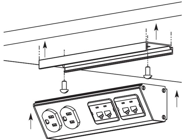
**NOTE:** Use No. 8 (5/16" [7.9mm] head size) flat head fastener or equivalent to secure mounting clip onto table surface (top or bottom).
