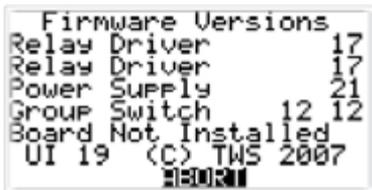
This screen lists all the boards in the panel and the firmware version of each. The example shown is a normal panel with 2 Relay Driver Cards (8 relays), a Power Supply and an optional Group Switch card. If "Board Not Installed" appears, but the board is physically installed in the panel, cycle power to the panel and check this screen again. If all installed boards still do not appear, advise Technical Support.
