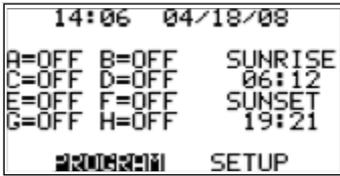
When the LP8 leaves the factory each relay is assigned to one of the 8 channels.
