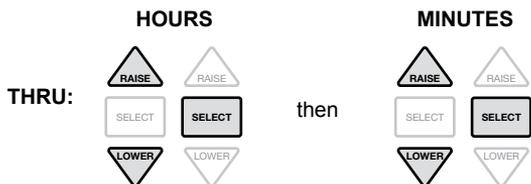
Repeat for second schedule OPEN/THRU period or continue to next step. If entering two on and off times for the day, enter the earliest on/off time on the first row. If only using one on/off time then enter it on the first row.
