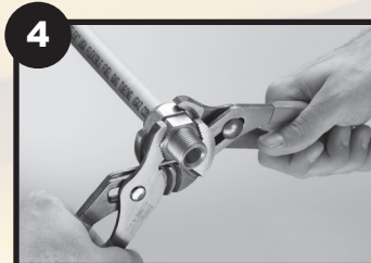
4 Tighten with wrenches until nut contacts body.
