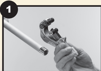
1 Cut tubing and remove PE coating to expose 4 corrugations.
