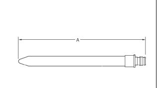
Uponor offers ProPEX<sup>®</sup> Copper Straight Stubs with PEX Lead-free (LF) Brass for use in hot and cold domestic potable water systems.<sup>1</sup> One end of the copper straight stub features the ProPEX LF Fitting for connections to Uponor AquaPEX<sup>®</sup> tubing with the end spun closed.
