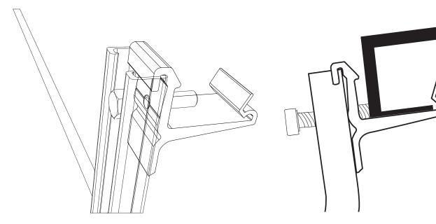
Material: 6105-T52, 6063-T5 Aluminum extrusion Ultimate Tensile: 38ksi Yield: 35ksi Finish: Mill Universal clamp to work with virtually every framed module
