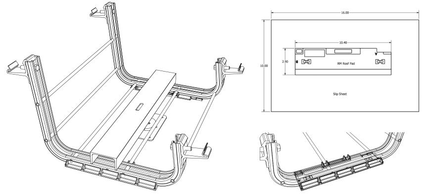
Material: TPE 70 Shore A Color: Black Thickness: 0.139" (base thickness) Width: 2.9" Length: 10.4" Quantity (per Ballast Bay): 2
