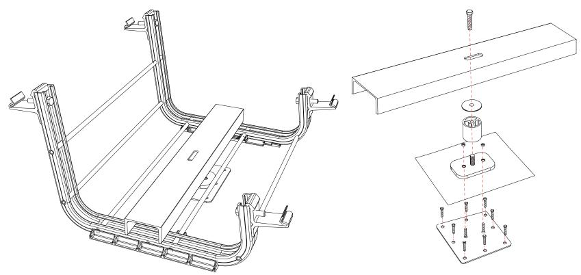
Material (clamp bar & standoff): 6105-T52, 6063-T5 Aluminum extrusion Material (Base Plate): 11 gauge thickness, Steel Allowable Lateral Load: 1200 lbs Standoff height: 1.7" Standoff Diameter: 1.66" Weight: 18 lbs Attaches to structure using Concealer Screws of various lengths
