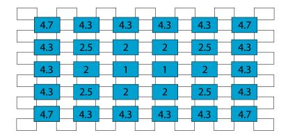
For a bay on the very perimeter edge of the array that supports 2 panels only contributes half of its weight to each panel it supports. The same goes for an interior bay that supports 4 panels, it only contributes <sup>1</sup>/<sub>4</sub> of its weight to each panel. After rounding up to whole blocks the resulting final ballast distribution is as follows:
