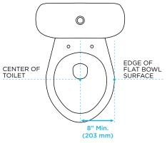
Minimum of 8 inches (203 mm) of open space from center of toilet to edge of flat bowl surface.
