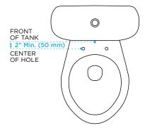
Minimum of 2 inches\*\* (50 mm) from front face of tank to the center of mounting holes.
