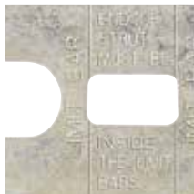
View window provides strut length safety zone for rough cuts versus precision cuts.
