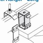
Illustration showing A854L with nut and bolt furnished to attach to fluorescent fixture. Use with E and H Series channel as well as A, B, C or D Series channel. Wt./C 51 lb.
