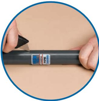
Step 1 consists of two cuts through the plastic to the substrate along the length of the conduit, approximately 1/2 in. apart and 3 in. to 4 in. in length. A third, perpendicular cut crosses the lengthwise parallel cuts.
