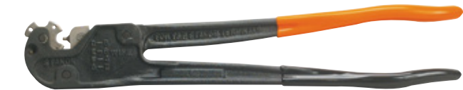
WT115A Toggle-type hand tool
