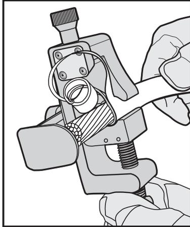
8B. For Mid-Span place a gloved hand against unibody frame while continuing to turn stripper clockwise.
