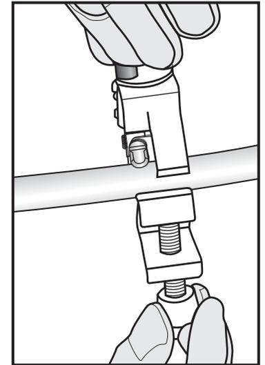
5. Engage V shape cable clamp by turning cable sizing thumb screw clockwise until cable is secured.
