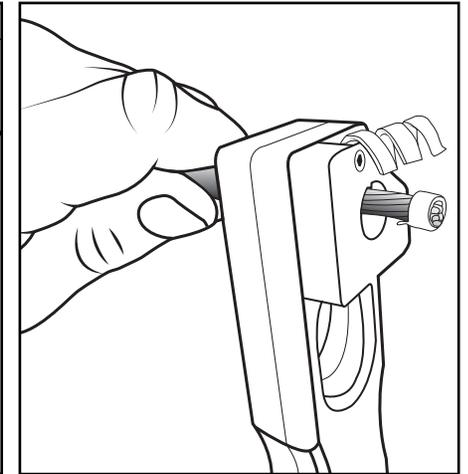
5. Once desired length of strip length is obtained, slide a finger of opposite hand against back side of stripper to stop advancement of the stripper. Continue to rotate until jacket material is rounded off.
