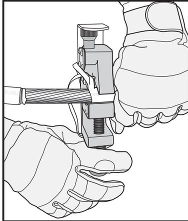
9. Release V shape cable clamp by turning counter clockwise to remove stripper.
