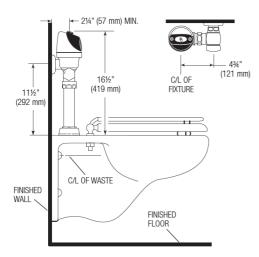
RESS-C units do NOT include a Valve Body, Supply Stop or Vacuum Breaker.
