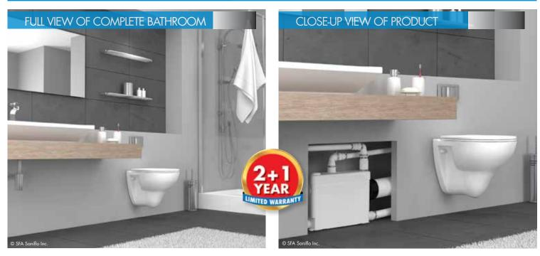
The Sanipack is a 1/2 HP pump system used to install a complete bathroom up to 15 feet below the sewer line, or even up to 150 feet away from a soil stack. It incorporates a macerating system which can handle human waste and toilet paper in residential applications.
