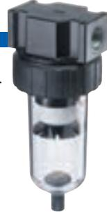
Amflo and Tru-Flate two-stage filters remove liquids, oil, water and large dust particles by centrifugal force, and small dust particles down to 40 microns by a porous element filter. Air line filters are vital to protect expensive air powered tools to keep them operating longer with greater efficiency.
