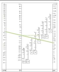
In the example for a design flowrate of 5GPM and design Δp 3psi handwheel position of 1.35 is determined for a 1" valve
