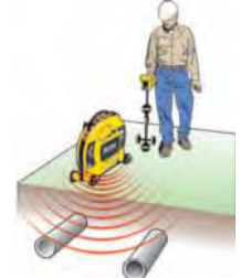
Induce a signal to locate utilities.
