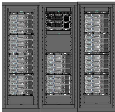
Example of 3 cabinet Pod with 40 2 RU servers distributed over 3 cabinets with 2 ToR switches in center cabinet requires 80 SFP+ cables with longest cable of 4m
