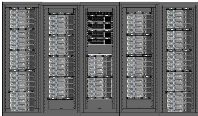
Example of 5 cabinet Pod with 80 2 RU servers distributed over 5 cabinets with 4 ToR switches in center cabinet requires 160 SFP+ cables with longest cable of 5m
