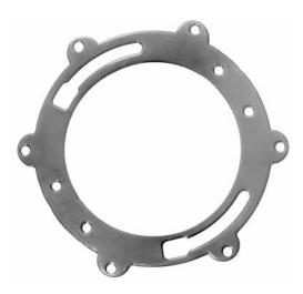
United States Patent 5,890,239 Unique screw tabs attach to wood or concrete. Plastisol coat provides corrosion protection. Slotted for 1/4" or 5/16" closet bolt. Old closet ring does not need to be present. Replaces any and all closet rings.
