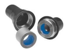
UNY and UNF unions are installed in threaded thick-wall conduit systems in hazardous areas. UNY unions are used to connect conduit to a conduit fitting, junction box, or device enclosure. UNF unions are used to connect conduit to conduit, or to provide a means for future modifications to the conduit system.
