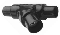
Sealing fittings restrict the passage of gases, vapors, or flames from one portion of the electrical installation to another at atmospheric pressure and normal ambient temperatures. They prevent precompression or "pressure piling" in conduit systems.
