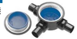
GUA series conduit bodies are installed within hazardous area locations to protect conductors in threaded rigid conduit, act as pull and splice boxes, provide access to conductors for maintenance and future system changes, act as mounting outlets for fixtures (with proper covers), or change conduit direction.
