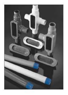
Specify OCAL-BLUE coating wherever the environment is corrosive... OCAL-BLUE is a dense polyvinyl chloride coating with a minimum thickness of 0.04" (40 mil) on the exterior and a chemically-cured blue urethane coating with a nominal thickness of .002" (2 mil) on the interior and over the hot dipped galvanized threads.
