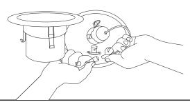
5 Align friction clips with recessed housing.
