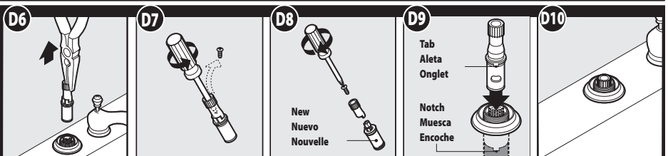
REASSEMBLY, REVERSE Steps D7-D1
