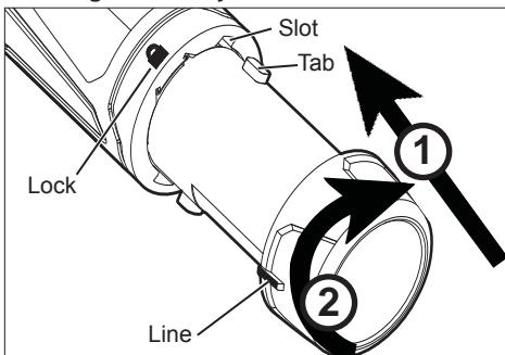
Line up the tabs on the battery with the slots in the tool opening. Slide the battery all the way into the tool. Turn the battery clockwise to lock it in place. The line on the battery will line up with the
