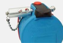
A 5/16" locking pin can be ordered to securely lockout receptacles that include the 'padlockable pawl' option. Alternatively the user can utilize a lock with a 5/16" shank. Locks with smaller shanks will NOT securely lockout a receptacle pawl.
