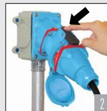
Pressing the pawl causes the DECONTACTOR to break the circuit. The plug is ejected to its rest position; its contacts are now dead.
