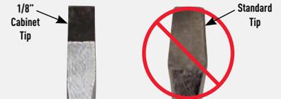
DSN20 terminal screws can be tightened or loosened with a 1/8" cabinet tip screwdriver. Meltric recommends Klein 608 Series or equal. The terminal screws on DSN20 devices cannot be properly accessed with a standard screwdriver.
