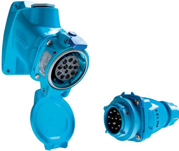
Effective immediately Meltric's PN12c devices will feature contacts that can be crimped or soldered. Previously the contacts could only be soldered. Each inlet and receptacle will now be supplied with 13 individual contacts (12 for the device and one extra if needed). The user can decide to install all 12 contacts or they can install less if 12 are not needed. Crimping offers advantages for some because it reduces installation complexity while still ensuring a quality connection.
