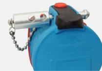
A 5/16" lockout pin can be ordered to securely lockout receptacles that include the 'padlockable pawl' option. Alternatively the user can utilize a lock with a 5/16" shank. Locks with smaller shanks will NOT securely lockout a receptacle pawl.
