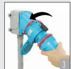
Rotating the 'dead' plug 30° counterclockwise closes the safety shutter and frees the plug to be withdrawn from the receptacle.
