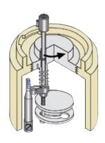
After depressing the pawl, the plug is rotated in a counter-clockwise direction. This frees the switching contact for operation and the release of the remaining spring tension causes a quick breaking of the contacts. The plug may now be removed, if desired.
