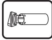
Attach pipe to vent by aligning clips on vent collar to slots on pipe and snap in place.
