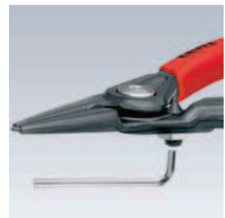
Style 3 / style 4: with adjustable opening restriction
