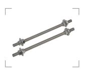
Pair of 11-1/2" long, 1/2" diameter zinc coated threaded rods with nuts and washers. Use with XTB02, STR04, R0L05 or R0L06 to elevate piping up to 14" overall height. Insert minimum 1" into Blox. 24 count bagged pairs, bulk packed cartons.
