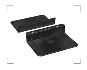
Pair of brackets secure Blox directly to roof surface. Brackets lock onto engineered mounting tabs with two #12x3/4" screws, then glue down into place with structural adhesive (ADH12/ADH12WH). Securing Brackets anchor the Blox into final installed position and protect against movement due to moderate wind, water, and snow loads.
