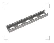
Mounts directly to Blox top in alignment trough with #14x1 sheet metal screws and washers or can be installed elevated with threaded extension rods (ROD03). Accepts strut clamps. 350lbs./158 kg max. static load with strut applied.
