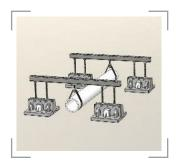
**082:** Two Blox Bridge with Underhung Piping
