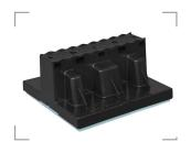
Polypropylene copolymer roof top support block engineered to support load directly attached with straps, clips or clamps, or the Blox easily adapts with accessories listed below. Includes on-board galvanized strap for short piping runs. Install every 7' along piping. 250lbs./113 kg max. static load single point loading. 350lbs./158 kg max. static load with strut applied. Bundled in convenient 8 pack totes.
