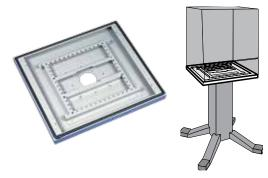
Closes off open bottom of sloped-front enclosures. Also fits COMPACT Series 4 Pendant Arm Flange Coupling Systems 80 and 80/140. The 14 gauge steel base has a stiffener framework attached to the inside and mounting holes that provide a rigid mounting means for 8.00 x 8.00-in. pedestal, pedestal extension, swivel tilt or angle adapter. Base has foam-in-place gasket and RAL 7035 textured light-gray polyester powder paint finish. Mounting hardware is furnished.
