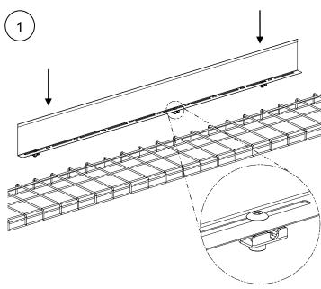
Loosely install 3 clips into desired slots of the Divider Wall and place onto Pathway.
