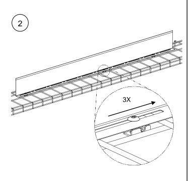
Slide the 3 clips onto the crosswires of the pathway.
