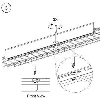
Tighten the screws to a torque of 5 ft/lbs
