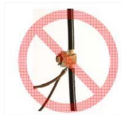
Figure 2 Terminating both sensor leads at the same point may result in inaccurate AVT results.
