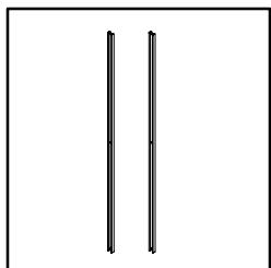
**NOTE:** Mounting channels may be assembled horizontally or vertically, as shown below. If mounting channels are to be used with DIN rails or grid straps, one channel nut for each DIN rail/grid strap must be inserted into each channel before channel is attached to enclosure, as shown below. If 36 inch or longer mounting channels are used with grid straps, the mounting channels must be inserted through the center slots of grid straps before attaching to enclosure, as shown.
