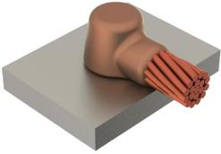
ERICO CADWELD Cathodic Connections are the preferred method of exothermically welding cathodic protection anode leads to pipes (steel or cast iron), tanks, and other structures. Cathodic protection systems are designed to prevent galvanic corrosion along a pipeline or in various structures. ERICO CADWELD Cathodic Connections use a special welding material alloy to minimize heat effect on the steel, which is especially important on thin wall and high stress pipes.
