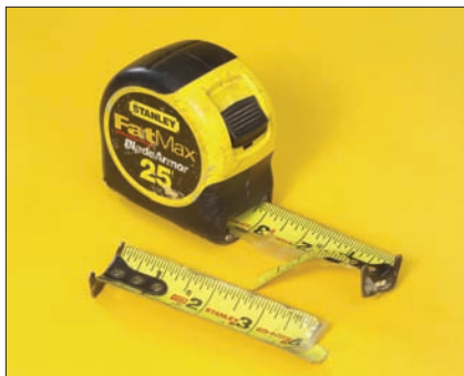
Torn or Damaged Blade
