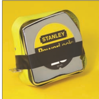
Broken Spring; Blade Will Not Retract
