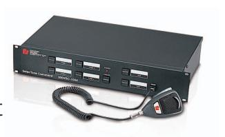
The Federal Signal Model 300VSC-1044SB SelecTone® Command Unit generates up to four tones or voice communications in a SelecTone system. The housing can be mounted in any standard 19" equipment rack. Four tones, auxiliary, test and cancel are controlled via an illuminated keypad. Voice transmission is activated by keying the optional desktop or hand-held microphone.
