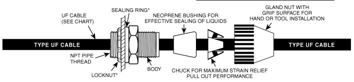
\*For knockout applications use T&B® 141 series locknuts and 5262 series sealing rings - purchase separately.
