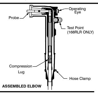
CAUTION: Lubricate test point cap and assemble tightly.
